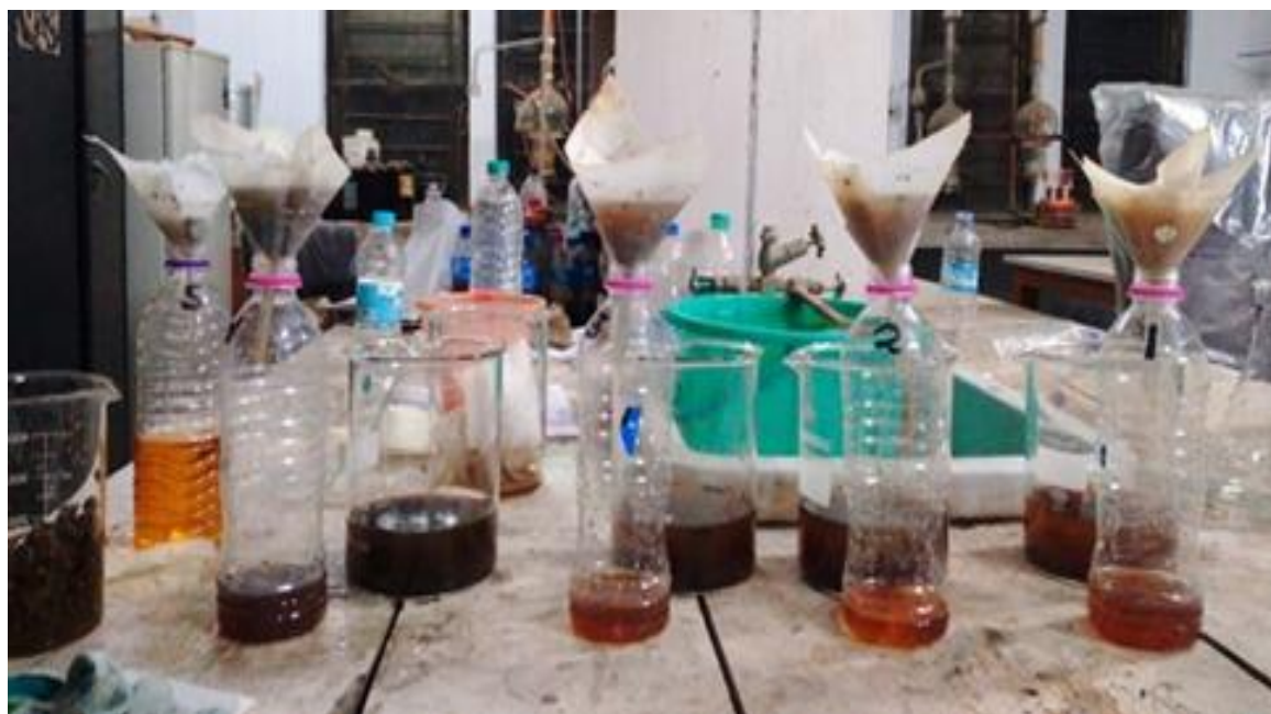
Fig. 15 Filtered compost liquid for heavy metal testing
