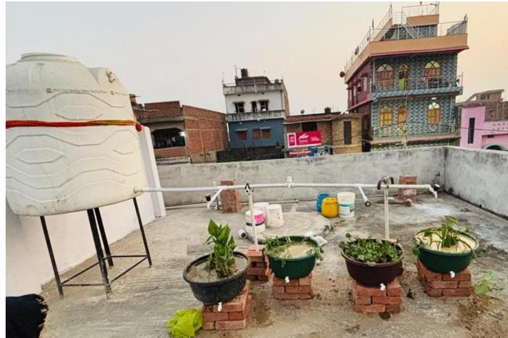
Figure 2. Vertical Flow Construction Wetland Prepared Model
