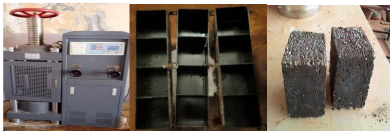
Figure 4 : compressive strength testing setup
