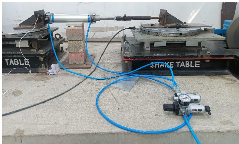
Figure 4 Real-time Photograph of Dynamic Testing of the Prototype PCAD Device through Shake Table Facility
