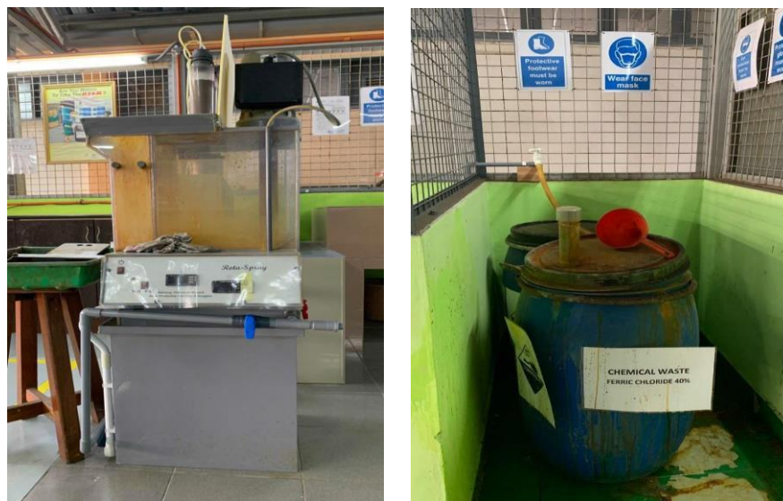
Figure 5: The installation of the new stop cork at the etching machine and piping line to the temporary disposal bin
