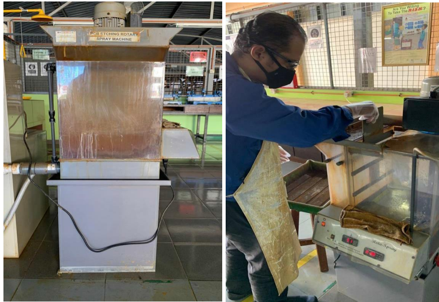
Figure 1: The PCB Etching Rotary Spray Machine and the Etching Process
