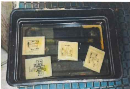
Figure 3.11.3 Removing Chemical from PCB Board
