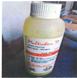
Figure 3.11.1 (PCB) Developer and is Acid Ferric Chloride
