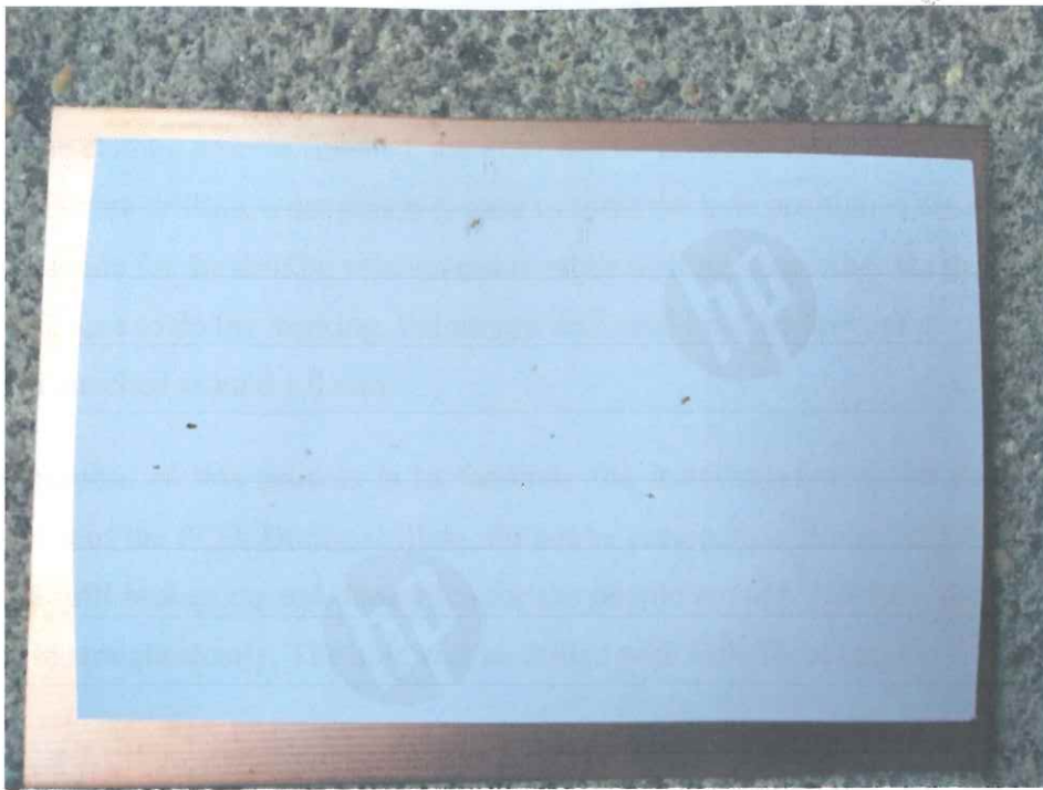
Figure 3.7 Step 3(Paste on the PCB Board using Iron)
