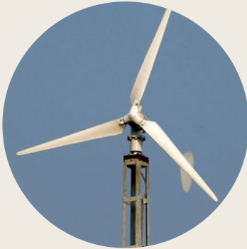
Figure 2.10 : Horizontal-axis wind turbines
