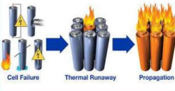
Fig.1: Risks of Thermal Runaway
