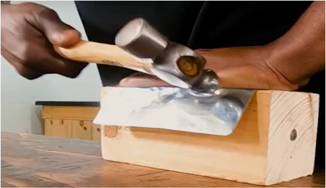
Figure 4 : Ball peen hammer used to shape metal. [8]
