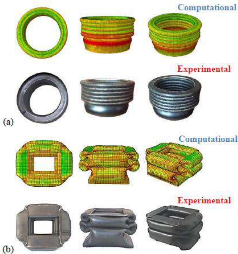
Figure 9: Final deformation and folding patterns observed in (a) cylindrical profile; and (b) columnar profile.
