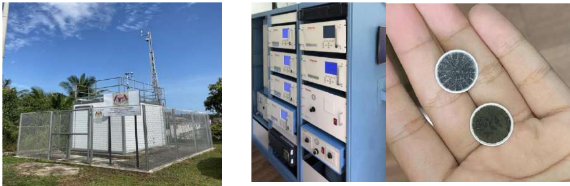
Figure 1. (a) Air Quality Monitoring Station, Indera Mahkota (b) Filter for Particulate Matter 2.5 & 10
