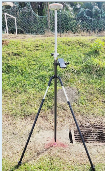
Rajah 3: Kaedah cerapan RTK GNSS
