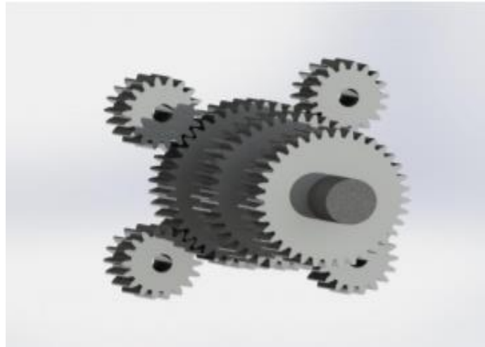
Figure 2 Basic Arrangement of Sun and Planet Gear Mechanism
