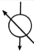
Water Cooled Condenser
