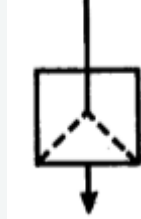
Reboiler (Kettle Type)
