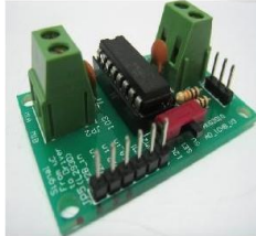
Figure 2 : DC Motor Driver
