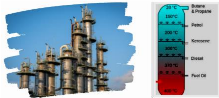
Figure 1.1 The Fractional Distillation Column and Its Separation Component
