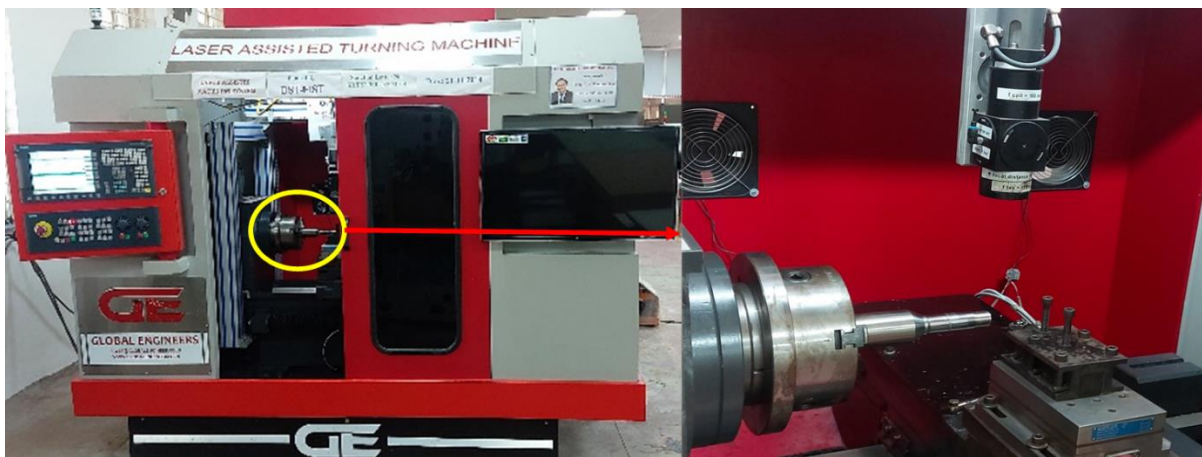
Figure 2. Laser assisted turning setup with enlarged view.
