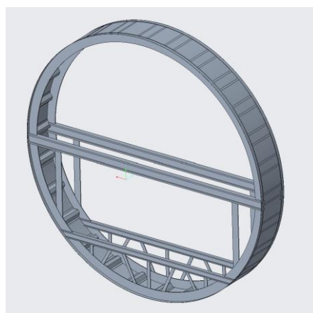
Fig. 3.1: Optimized Fuselage cross section model
