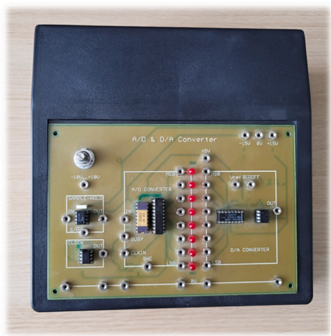
Fig. 4. Exchangeable functional board with ADC and DAC circuits.
