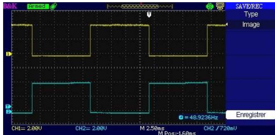
Figure 10. Waveforms of the A-L and B-L signals from the DC-AC converter.
