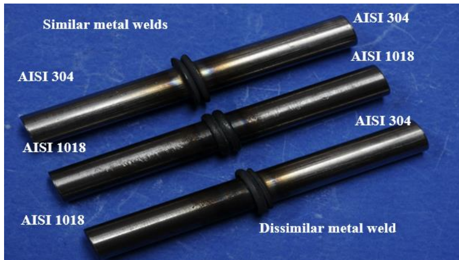
Figure 4 Specimens of Similar and dissimilar metal friction welds
