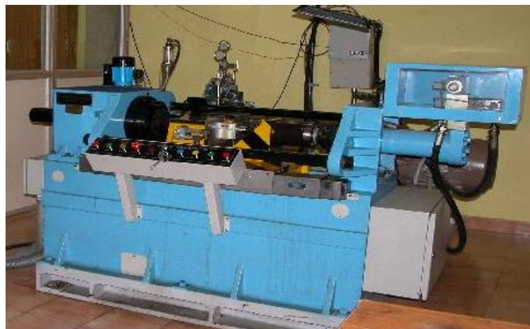
Figure 2 Continuous drive friction welding machine
