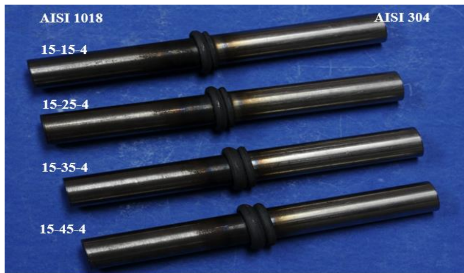
Figure 4 Specimens of Similar and dissimilar metal friction welds
