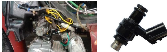
Figure 1. Actual image of 2 CNG nozzles installed on the intake manifold (left) and nozzle shape used (right)
