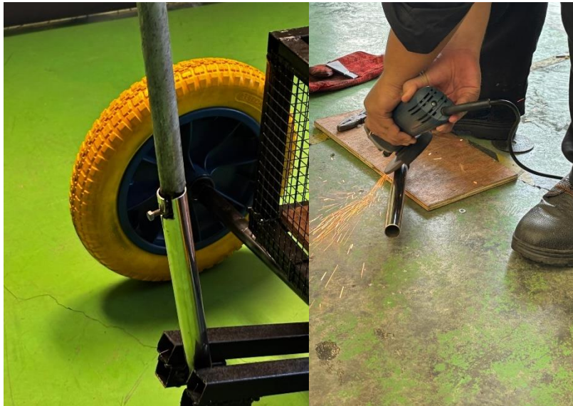
Figure 4.6 The progress of handle for trolley. Cutting the steel to be used as a spike protector
