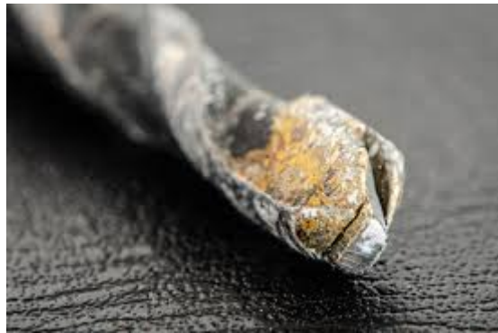
Figure 2.3: Damaged drill bit
