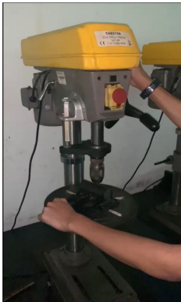
Figure 1.2: Clamp in Polytechnic Banting Machining Workshop for drilling process
