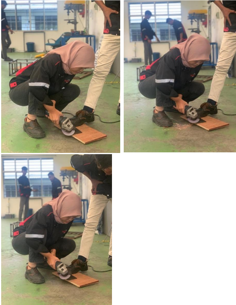
Figure 4.7: The surface Of The Central Frame Was Ground To Smooth Out Any Rough Areas
