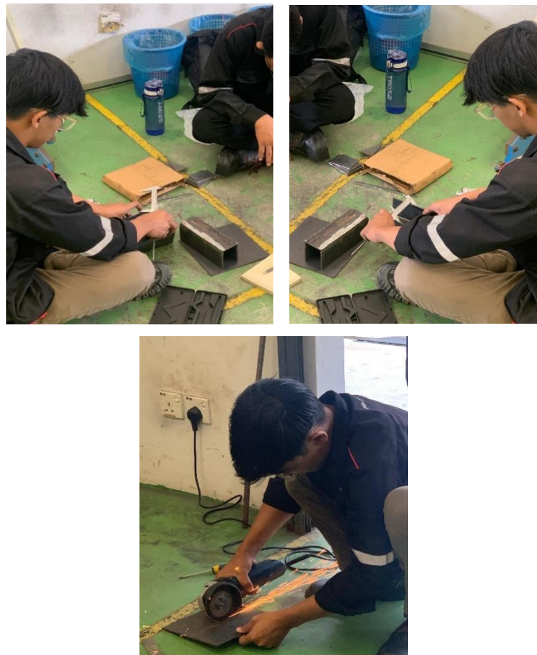
Figure 4.5: Metal Pieces For the Central Frame Were Measured And Cut According To The Design Requirements
