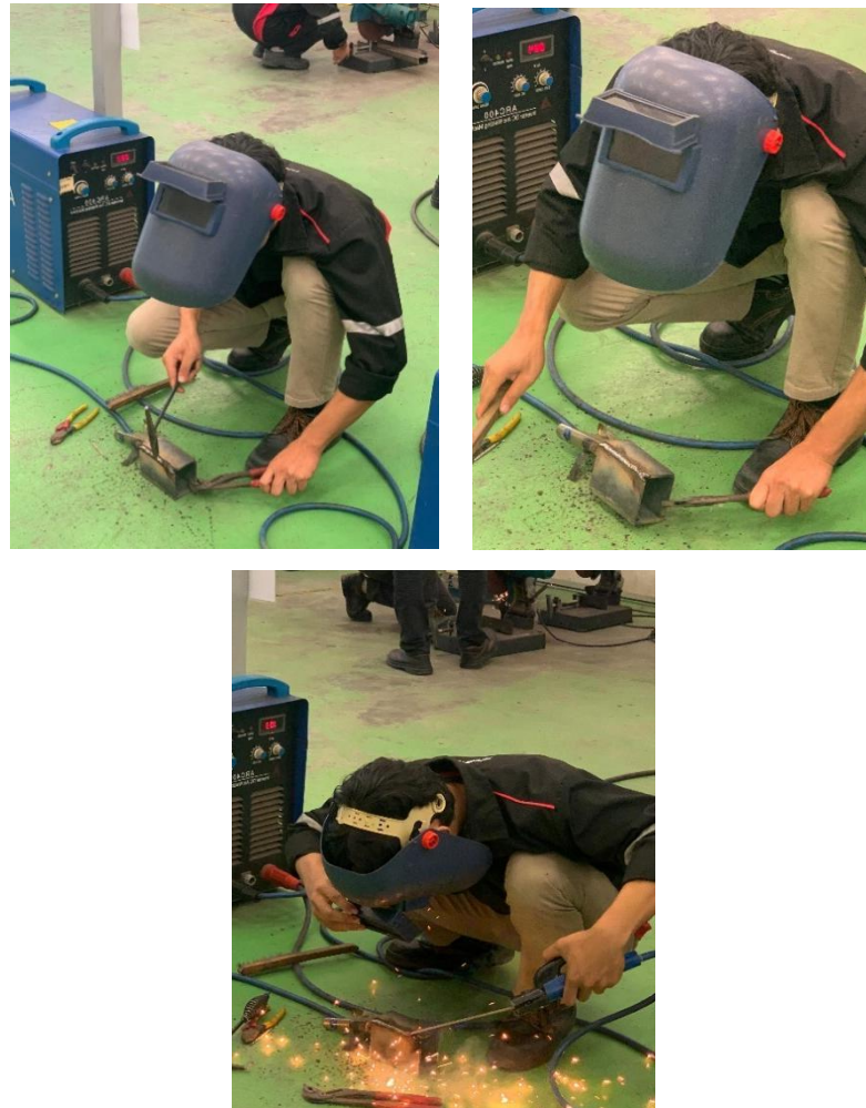
Figure 4.3: Cut Metal Pieces Were Welded Together To Build Foundation Of The Automatic Vice
