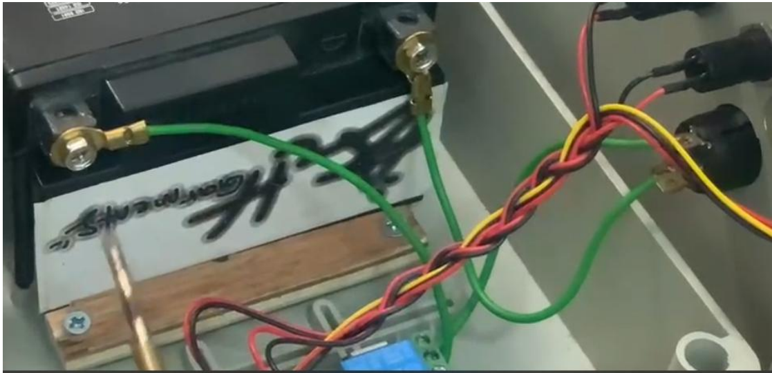
Motor Battery That Is Connected With Modular And Main Power Switch On The Cover
