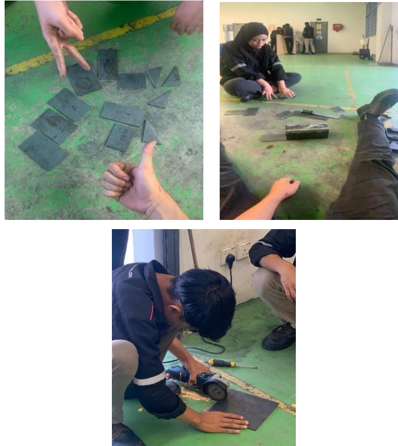
Figure 4.2: The metal plate for the base structure was measured accurately and cut to the specified size.
