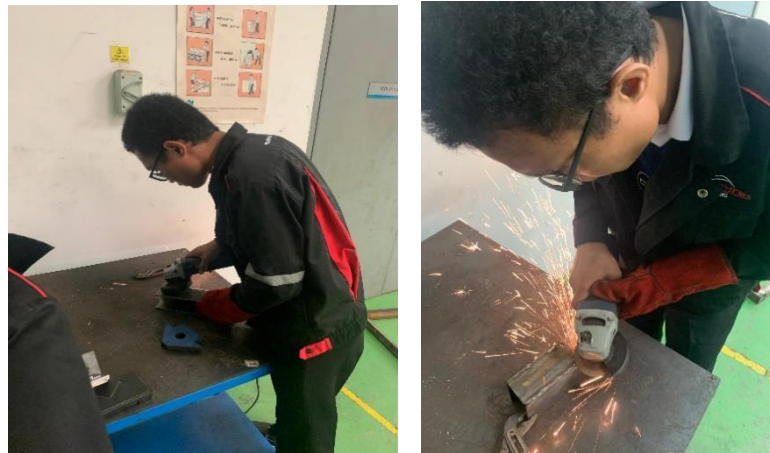
Figure 4.4: The surface Of The Body Structure Was Ground To Smooth Out Any Rough Areas
