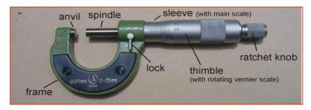
Figure 1.2: Micrometer screw gauge
