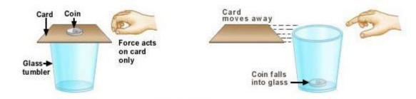
Experiment to demonstrate inertia
