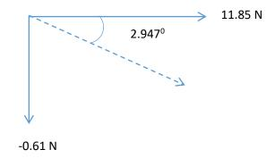
a) Determine resultant force,  $F_R$  for the system of forces shown in the Figure below.
