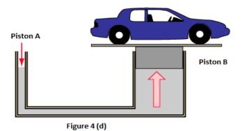
c) Figure 2 shows a hydraulic lift with a force  $F_1$  acting on a circular piston with an area of 0.02 m<sup>2</sup>. The pressure generated is transmitted through a liquid to a second piston with area of 0.12 m<sup>2</sup>. Calculate the minimum force  $F_1$  which need to be applied so that a load of 5000 N is lifted.
