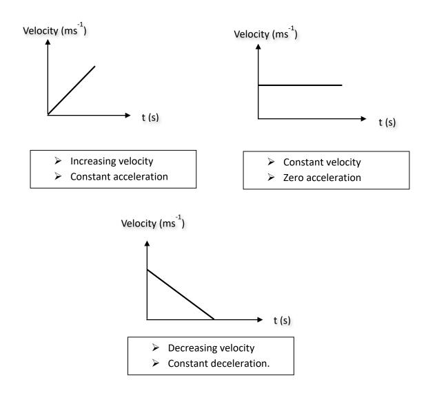
Figure 2.1 shows the combination of uniform acceleration, velocity and deceleration.
