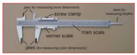
Figure 1.3: Vernier calipers
