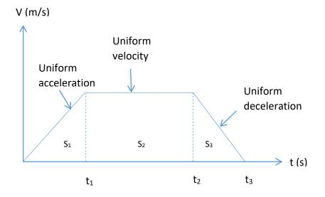
A monorail starts from rest and accelerates at constant acceleration of 5ms<sup>-2</sup> for 8 seconds. The monorail then travels at a constant velocity for 10 seconds. The brakes are then applied and the monorail stops in 5 seconds.
