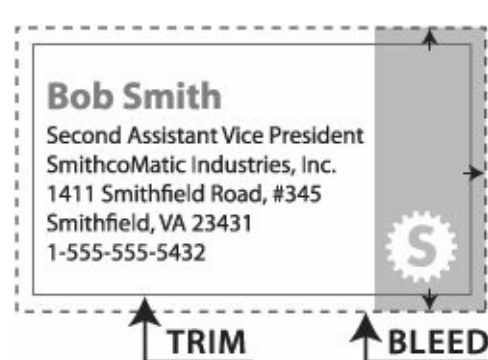
Figure 3.5. Extending artwork to provide bleed. The document is built to the correct final trim size, and the bleed extends beyond the trim.
