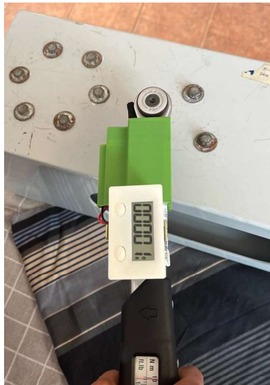
Figure 7 Final product of the digital torque wrench with built-in counter and attached 3D printed casing.
