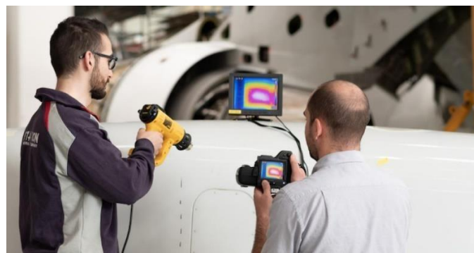
Figure 1.6: Traditional way Inspection using Thermography Testing.
