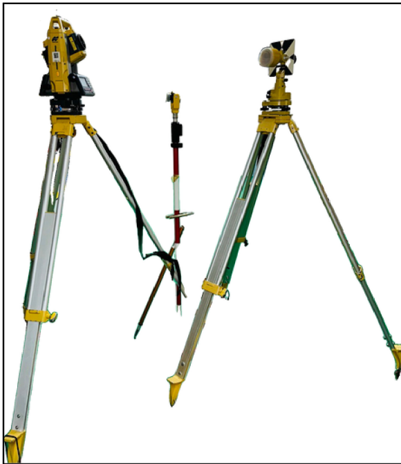
Figure 3.0: Basic Survey instrumentation; Total Station, Prism and Mini Prism
