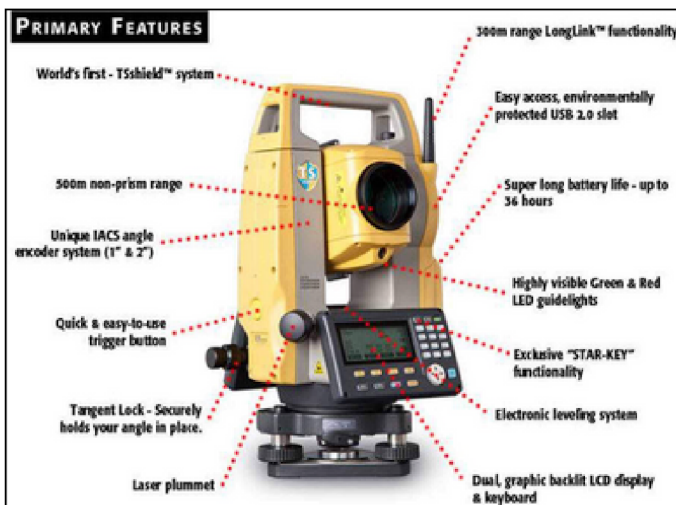
Figure 3.1: Total station parts model Topcon GTS
