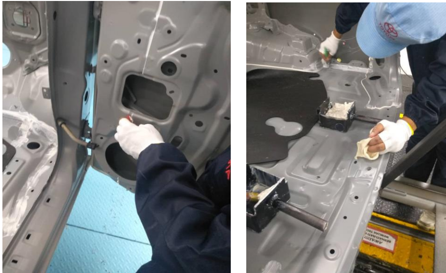
Figure 5.6: Finishing process or spatula process
