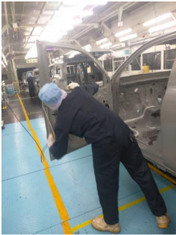
Figure 2.0: Process apply sealer line on the door
