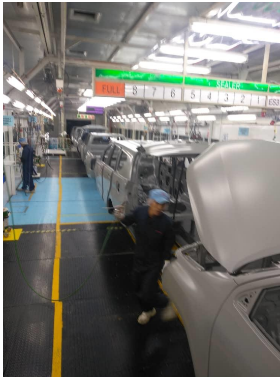
Figure 4.1: Sealer production line
