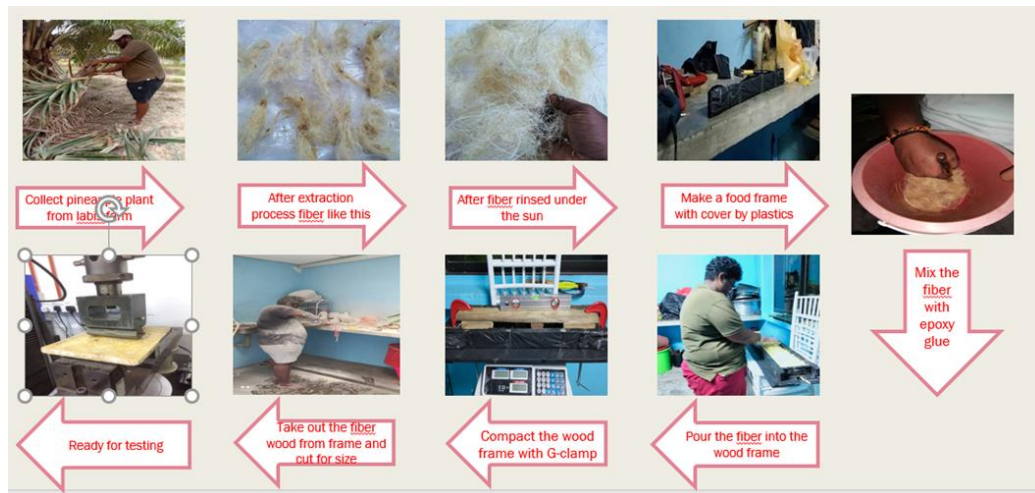
Figure 3.1 Procedure Preparation of Pineapple Fibre Wood
