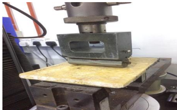
Figure 3.3 : Flexural Testing on Pineapple Fibre Wood And Normal Fibre Wood.
