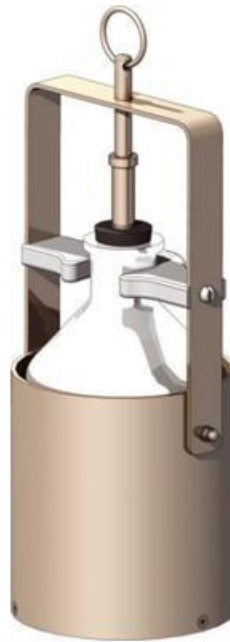
Rajah 2.3 : Weighted Bottle Sampler
