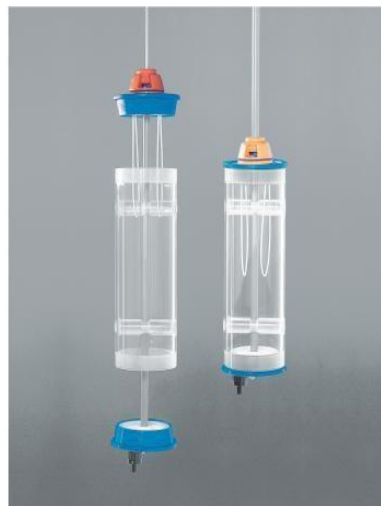
Rajah 2.2 : Kemerrer Water Sampler
