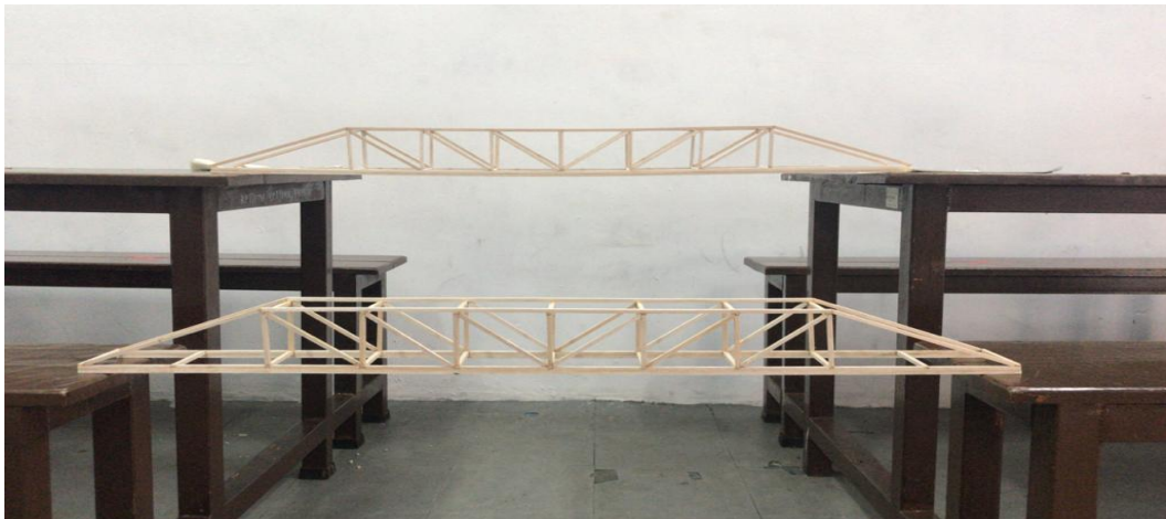
Figure 4.1(c): Pratt Bridge Model
