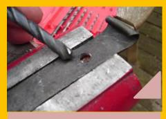
Pilot hole will allow you to centre the tip of the larger diameter tool and then accurately drill your final size hole. This often keeps the larger tool from jumping all over the surface when it first touches the material.
