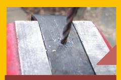
Drill a small pilot hole on the spot with a smaller bit if you will be drilling a large hole.
