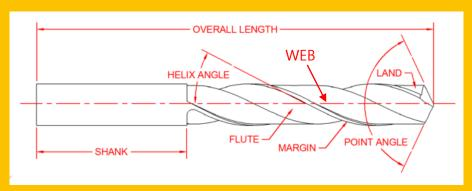
**FLUTES** – In order to create cutting lips, enable chip removal, and allow cutting fluid to reach the cutting lips, helical or straight grooves were cut or created into the drill's body.
