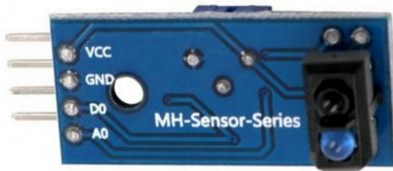
FIGURE 13: SINGLE CHANNEL IR SENSOR (FOR LINE FOLLOWER)
