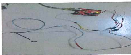
Figure 2.2(b): RTD connected to the input of the microcontroller
