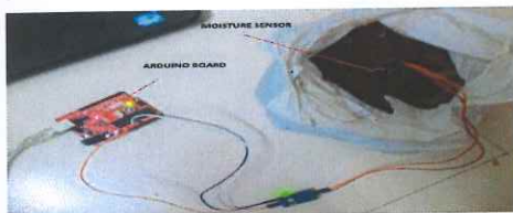
Figure 2.2(a): Moisture sensor connected to the input pin of the microcontroller
