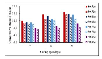
Fig. 5. Compressive strength results
