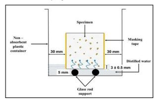
Fig. 3. Sorptivity test setting up
