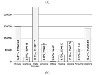
Fig. 8. Average value of energy consumption (MJ) and percentage (%) for (a) standard production line, (b) alternative production line
