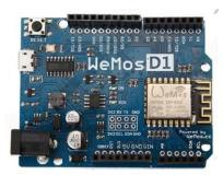
Fig. 4. WeMos D1 ESP8266 base board
