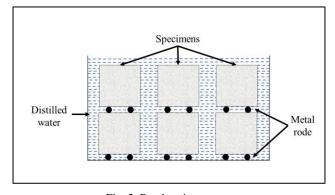
Fig. 2. Pond curing set-up
