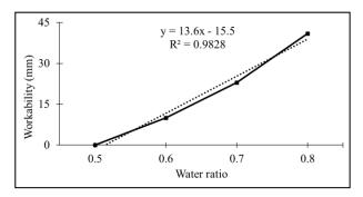
Fig. 1. Slump test results
