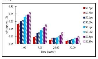
Fig. 6. Sorptivity test results
