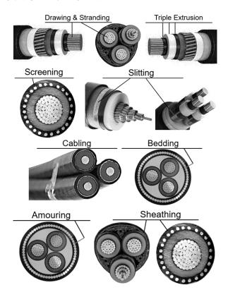
Fig. 1. Cable structure for the studied cable
