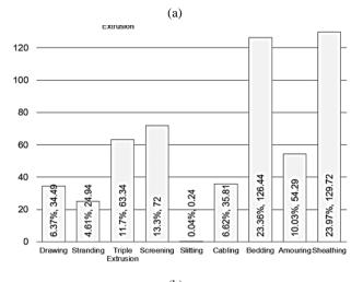
Fig. 7. Average value of time required (Hours) and percentage (%) for (a) standard production line, (b) alternative production line
