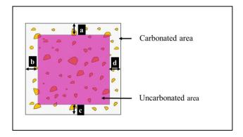
Fig. 4. Carbonation measurement depth
