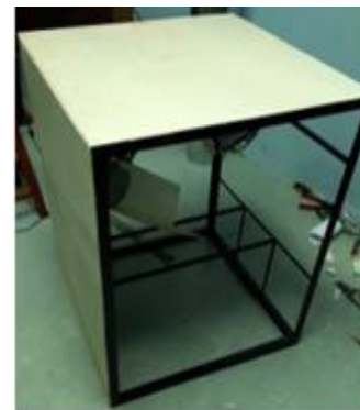
Fig. 10. Installing the plywood to the frame
