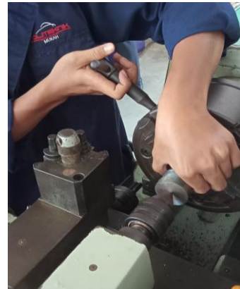
Fig. 2. Existing tightening process (without jig)
