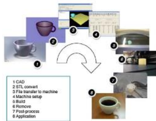
Fig. 3. Generic process of CAD to part, showing eight stages (Gibson, 2021)
