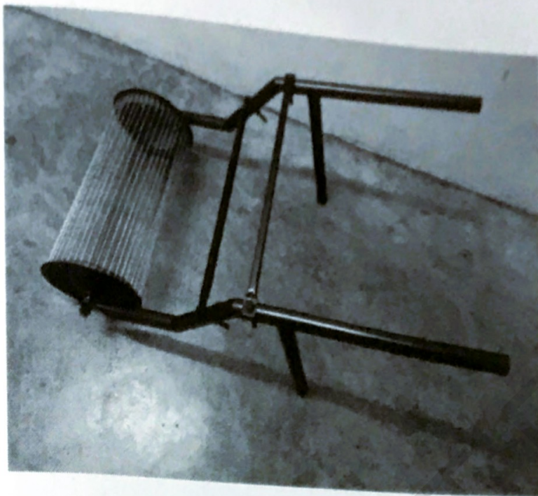
The complete design of oil seed roller collector
