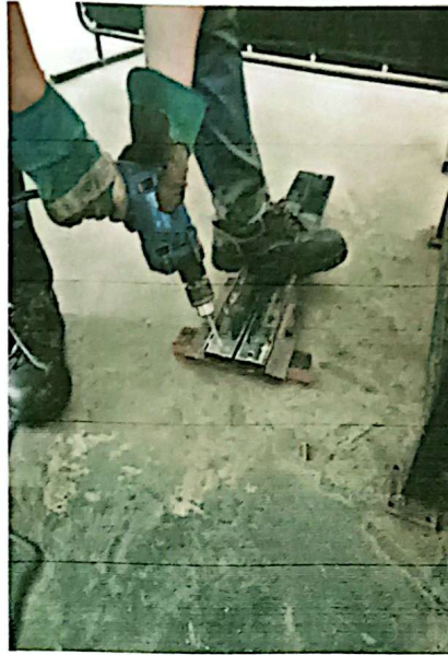
Figure 3.12 Drilling process of hollow bar
