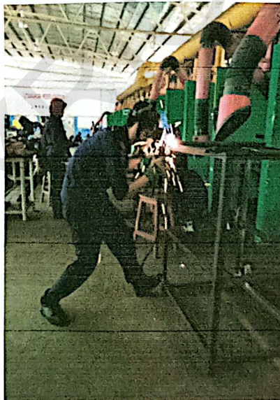
Figure 3.11 Arc welding of body frame
