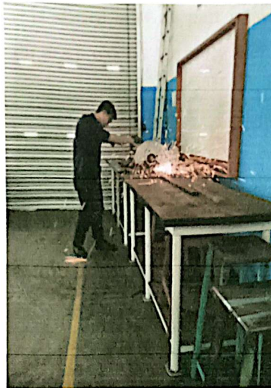
Figure 3.10 Cutting Process of angle bar
