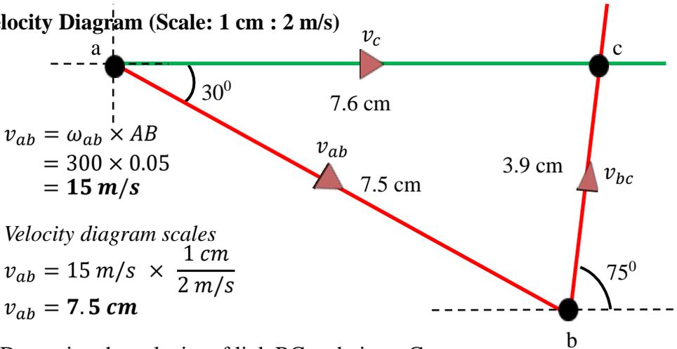
$$v_{ab} = \omega_{ab} \times AB$$
