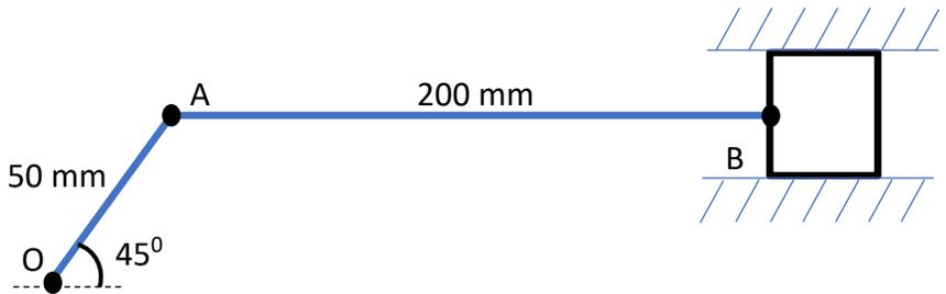
$$v_b = 1.11 \text{ m/s}; \quad \omega_{ab} = 5.55 \text{ rad/s}$$
