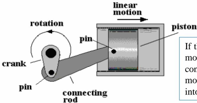
If the piston is forced to move, linear motion is converted into rotary motion and the force into torque
