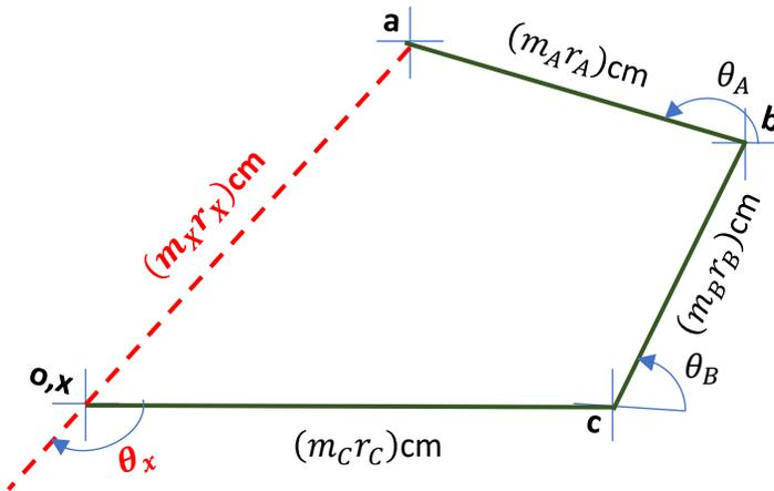
**Step 4 :** Convert balancing force from cm to kgm (refer scale), **determine;**
