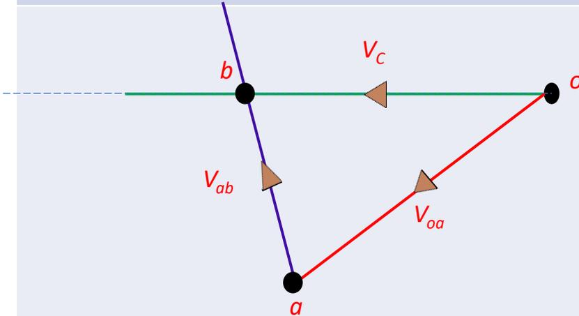
✓ Determine the piston's axis and then start drawing the diagram from a fix point
