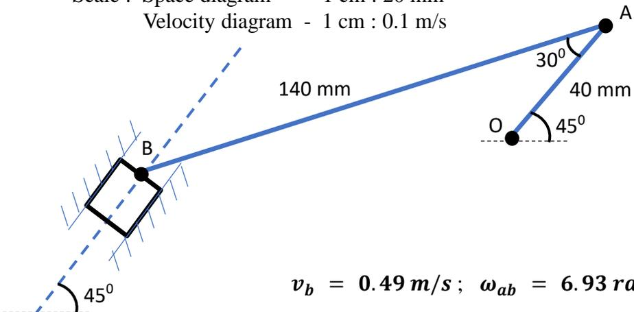
$$v_b = 0.49 \text{ m/s}; \quad \omega_{ab} = 6.93 \text{ rad/s}$$
