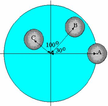
**Ans:  $m_x = 2.4 \text{ kg } \angle 152^\circ \text{ cw from A}$**
