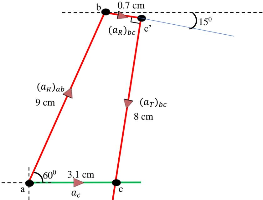
e) Determine the angular acceleration of link BC and piston C
