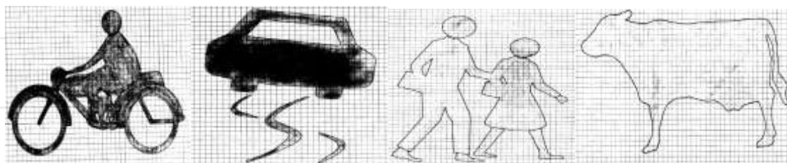
Figure 2-16: Symbol Templates (Source: Jabatan Kerja Raya, MANUAL ON TRAFFIC CONTROL DEVICES STANDARD TRAFFIC SIGNS, JKR/J(Rb) 0001/80)
