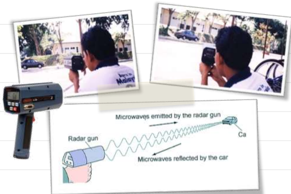
Figure 1-7: Spot speed study using radar meter
