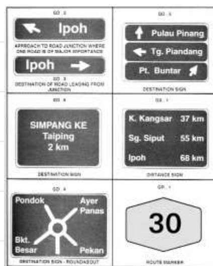
Figure 2-13: Guide Destination/ Guide Distance Signs and guide route marker (Source: Jabatan Kerja Raya, MANUAL ON TRAFFIC CONTROL DEVICES STANDARD TRAFFIC SIGNS, JKR/J(Rb) 0001/80)
