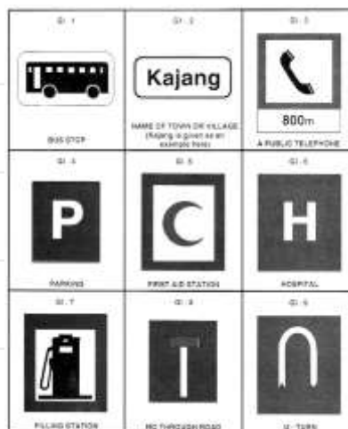
Figure 2-12: Guide Information Signs (Source: Jabatan Kerja Raya, MANUAL ON TRAFFIC CONTROL DEVICES STANDARD TRAFFIC SIGNS, JKR/J(Rb) 0001/80)
