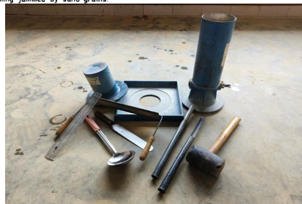
Figure 1 — Small pouring cylinder for the determination of the density of fine and medium-grained soils
