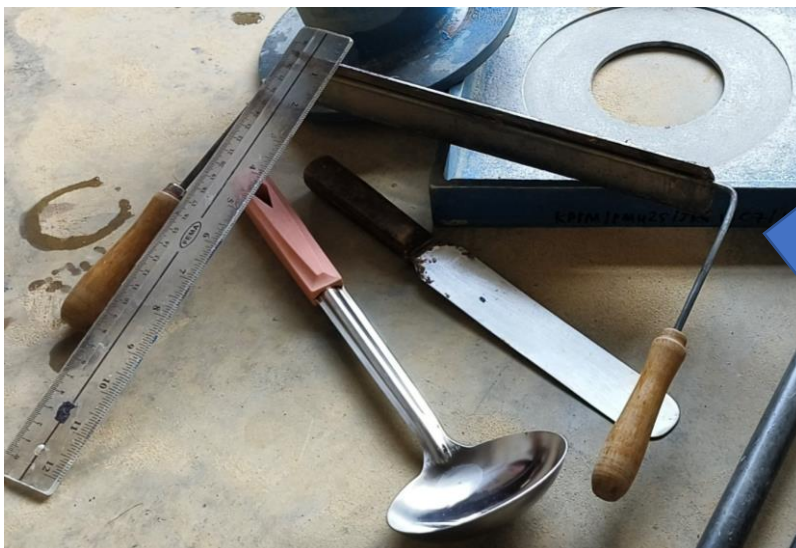
Figure 2 — Scraper for levelling surface of soil
