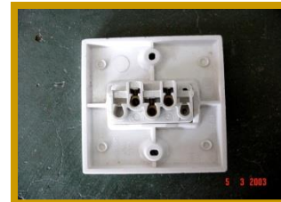
Single Pole Two Way Switch
