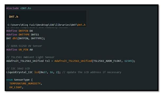
Figure 3.19: Arduino Coding for Sensors in Arduino IDE Software
