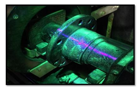
Figure 2.4: Magnetic Particle Suspended at Defected Area (Google n.d.)
