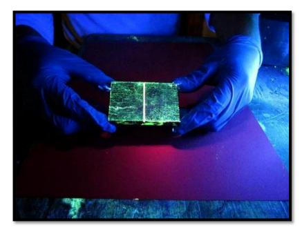
Figure 2.7: Fluorescent Penetrant Testing (Google n.d.)
