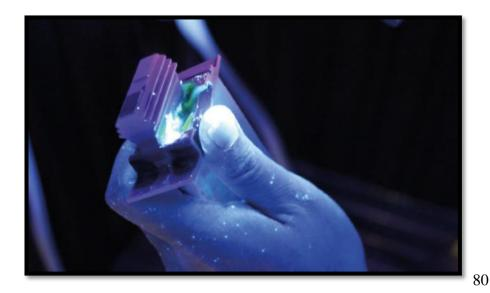
Figure 1.1: Fluorescent Penetrant Testing (Source Advanced Engineering: Google)
