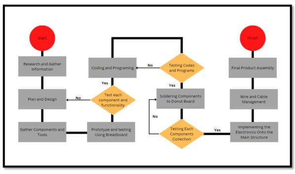
Figure 3.7: Electronic & Programing Flow Chart
