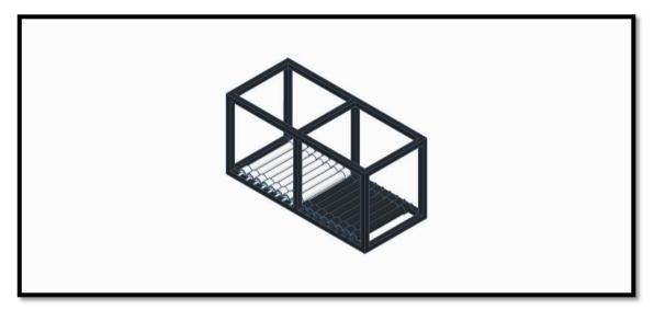
Figure 3.17: Isometric View of Roller Conveyor with The Mainframe Structure
