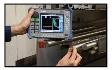
Figure 2.2: Conducting an Ultrasonic Testing (Google n.d.)
