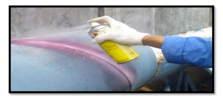
Figure 2.5: Liquid Penetrant Testing (Google n.d.)
