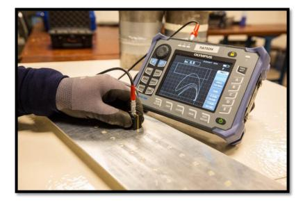
Figure 2.3: Conducting Eddy Current Testing (Google n.d.)
