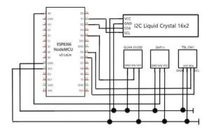
**Figure 3.18: Schematic Drawing of the Electronics construction**
