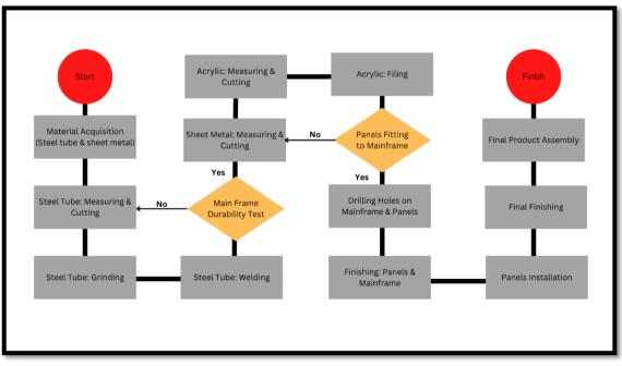
Figure 3.5: Product Structure & Finishing Flow Chart
