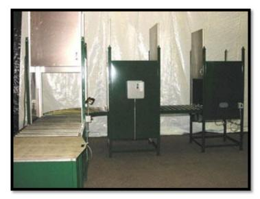
Figure 2.8: "L" Layout of Liquid Penetrant System (NDT Supply.com, Inc, n.d.)
