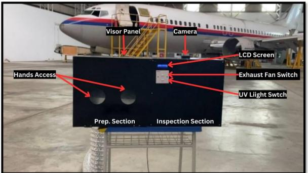
**Figure 4.1: Front View of Finished Product with Labels**
