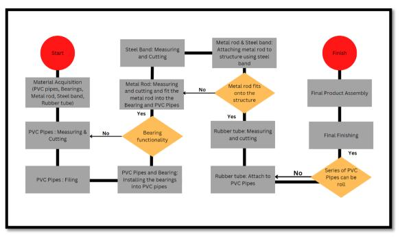
Figure 3.6: Conveyor Roller Flow Chart
