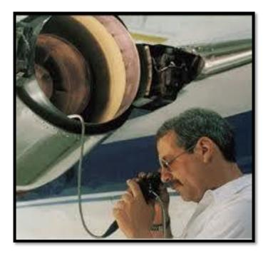
Figure 2.1: Visual Inspection by Borescope (Google n.d.)
