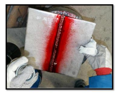
Figure 2.6: Dye Penetrant Testing (Google n.d.)
