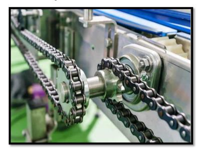
Figure 2.16: Chain and Sprocket System (Google n.d.)
