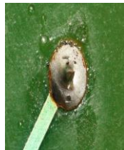
Cold Solder Joint
