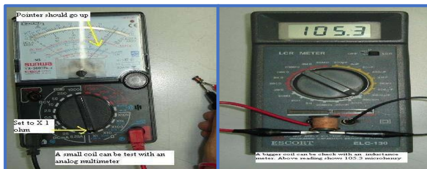
Figure 3.5: Testing inductor using multimeter
