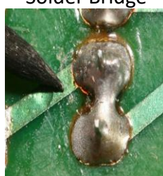
Figure 1.10: An example of bad soldering
