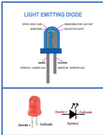
Figure 3.12: LED symbol and construction diagram
