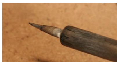
Properly Tinned Soldering Iron Tip
