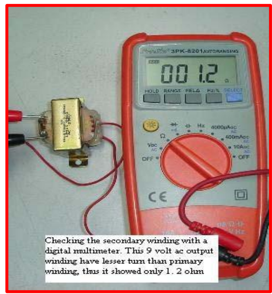
Figure 3.18: Testing linear transformer using multimeter
