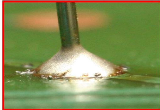
Figure 1.9: An example of good soldering
