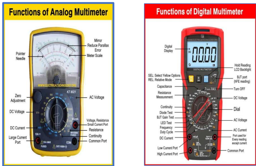
Figure 2.13: Analog And Digital Multimeter Features
