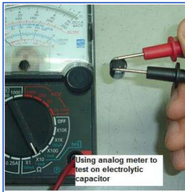
Figure 3.22 Testing capacitor using an analogue multimeter
