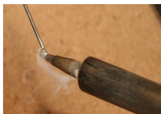
Apply Solder to Soldering Iron Tip
