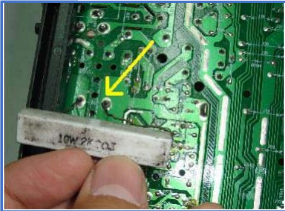
Figure 3.20: Discharge Capacitor Using Resistor
