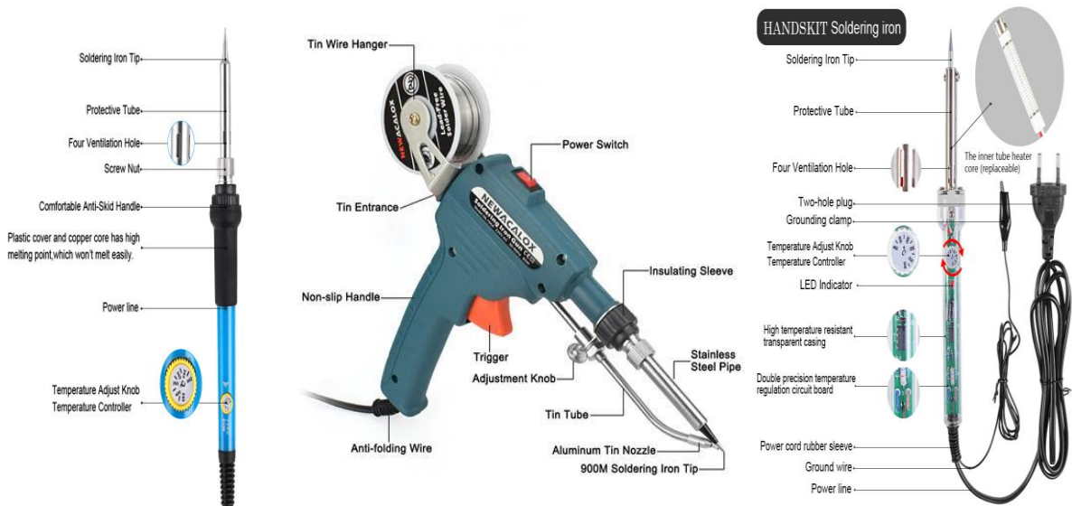
Figure 1.6: Soldering iron features
