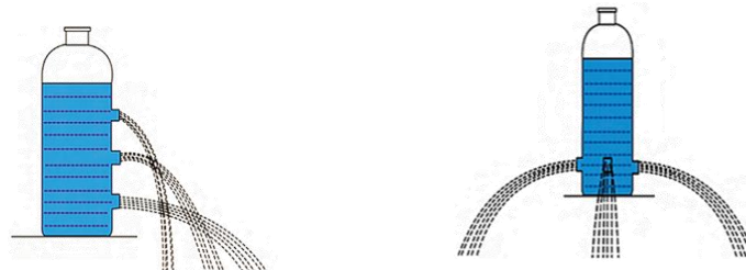
Nozzles at different depth Nozzles at the same depth
