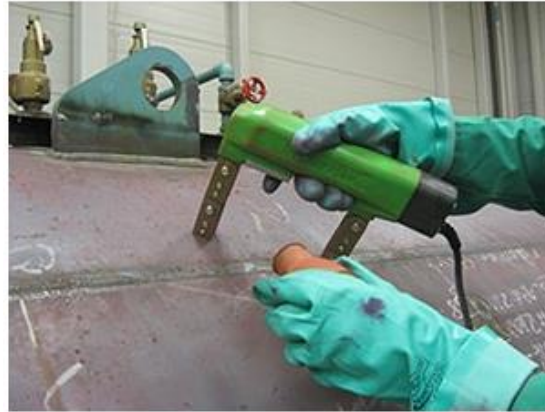
Figure 10 External longitudinal seam being checked with MPT using an AC yoke with dry powder [8]
