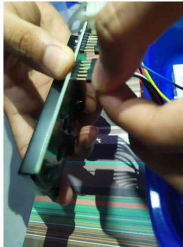
Figure 3.6 : The wire is connected to the LCD
