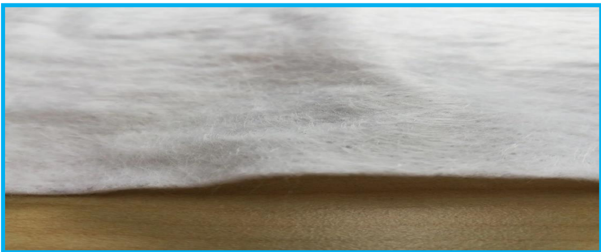
Figure 2.2: Close look-up of non-woven geotextile
